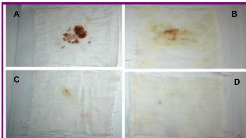
Figure 12. Washing performance of protease in presence of detergent (Surf excel). A. Cotton cloth stained with blood; B. cloth stained with blood and washed with distilled water only; C. cloth stained with blood and washed with detergent only; D. cloth stained with blood and washed with the detergent and enzyme solution.
